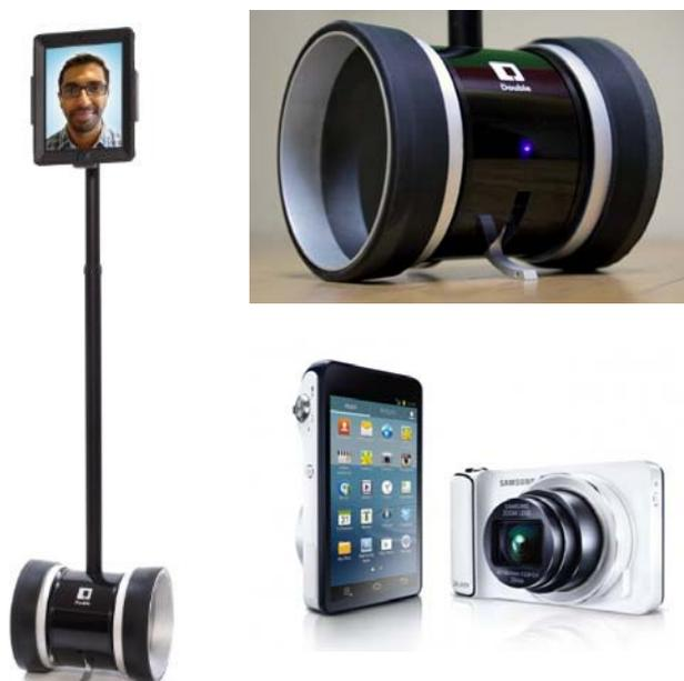
**Figure 1.** Low cost devices. A robotic foot for the iPad and the Samsung Galaxy camera. The first from double robotics, the second with an Android OS that allows to use Ubuntu and also the GNU-health for mobiles devices using Tryton.
