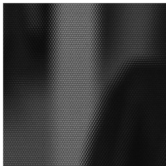
**Figure 3.** Raw image. Detail of the density and pixel structure on LFC (light field cameras).
