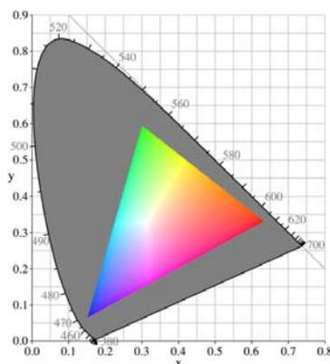
**Figure 2.** Triangle showing the classic color gamut CIE 1931 represented in the RGB computer monitors.
