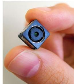
**Figure 6.** Left detail of the microlenses from Pelican Imaging Corporation. Right . Taken from [11]. Toshiba miniature lightfield camera (LFC) module for smartphones and tablets.Taken from [12]
