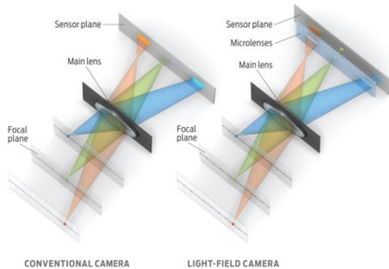
**Figure 4.** Microlenses galore. Comparison between a conventional camera (left) and the LFC (right). In the conventional camera the light from the focal plane (green) is the one focused in the image plane, the rest are out of focus points (blue and orange). The LFC projected the 3 planes into a microlenses array that focused the image in the sensor plane therefore the out of focus image is digitally synthesized. Taken from [7]
